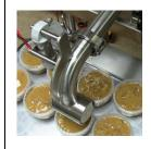
Injection nozzle double, for semi-liquid products, soft paste, aerated products
