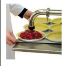
Handgun nozzle, for liquid, semi-liquid products, soft paste, heavy paste, aerated products
