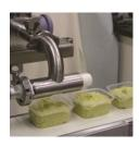
Rotary cut-off nozzle, for semi-liquid products, soft paste, heavy paste, aerated
