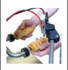
Double injection/fill attachment, to attach injection needles/pastry tips/tubes
