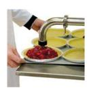
Handgun nozzle, for liquid, semi-liquid products, soft paste, heavy paste, aerated
