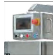
MULTIFUNCTIONAL DISPLAY WITH TOUCH SCREEN AND USB CONNECTION. PAD ON MOVABLE ARM / MULTIFUNKTIONSDISPLAY (TOUCH SCREEN, USB, SCHWENKBAR)
